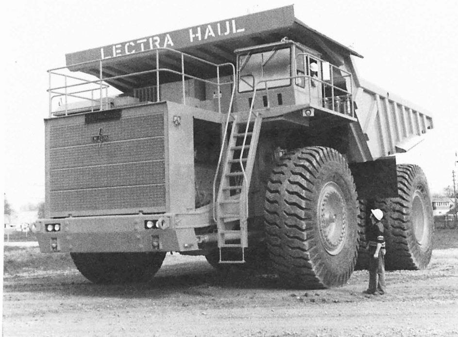
UNIT RIG LECTRA HAUL M-200 WITH A 2450 HP ENGINE
