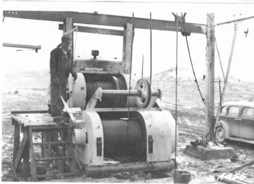
U-20 Telescoping Mast With a U-17/U-19 well serving unit
