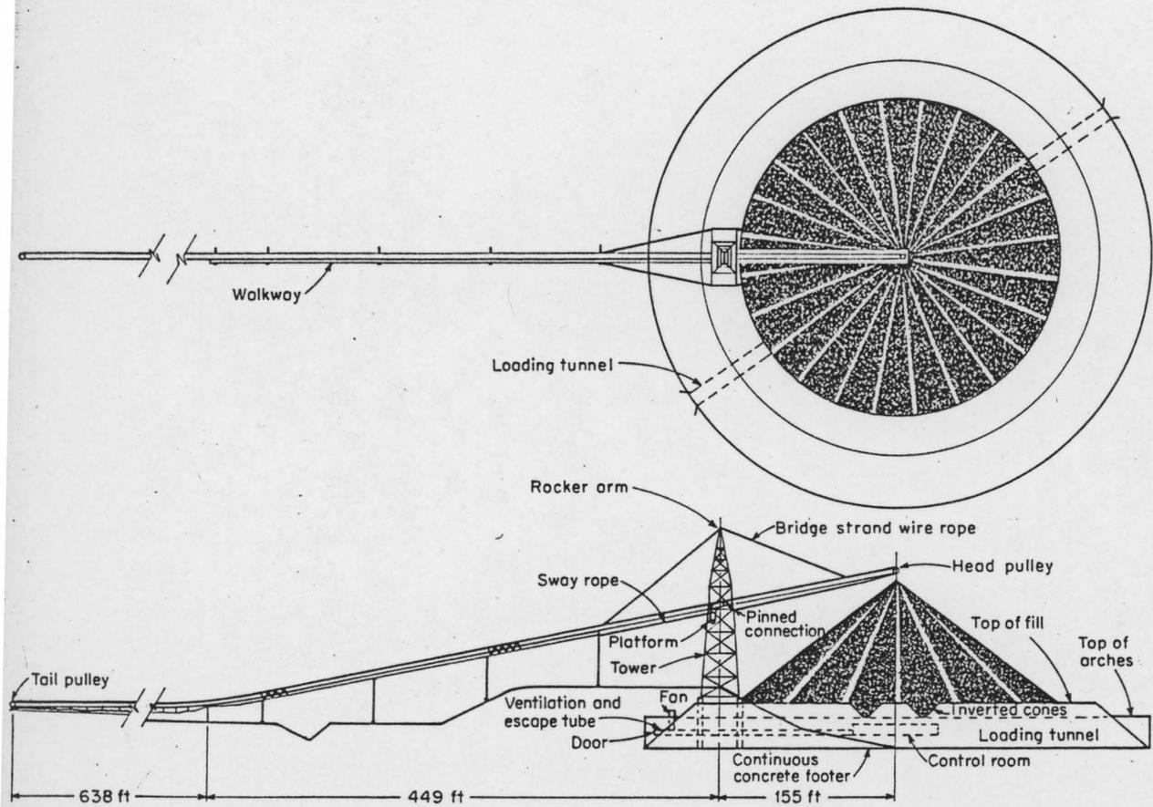
General arrangement of Sunnyside's high-capacity unit-train loading facility details major features, including the conveyorway, tunnel, steel cones, loading gates and tower. More than 400 tons of steel was used.
