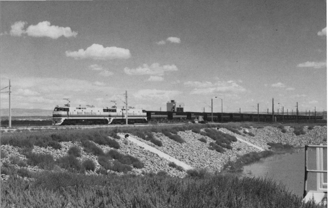
The concept is simplicity itself. At one end of a point-to-point layout is a coal mine, at the other an electrical generating plant. In between, an archtypical unit train. Seen here at the Bonanza end are the coal pile and handling facilities with the essential train ready to shuttle back for more of the same.
