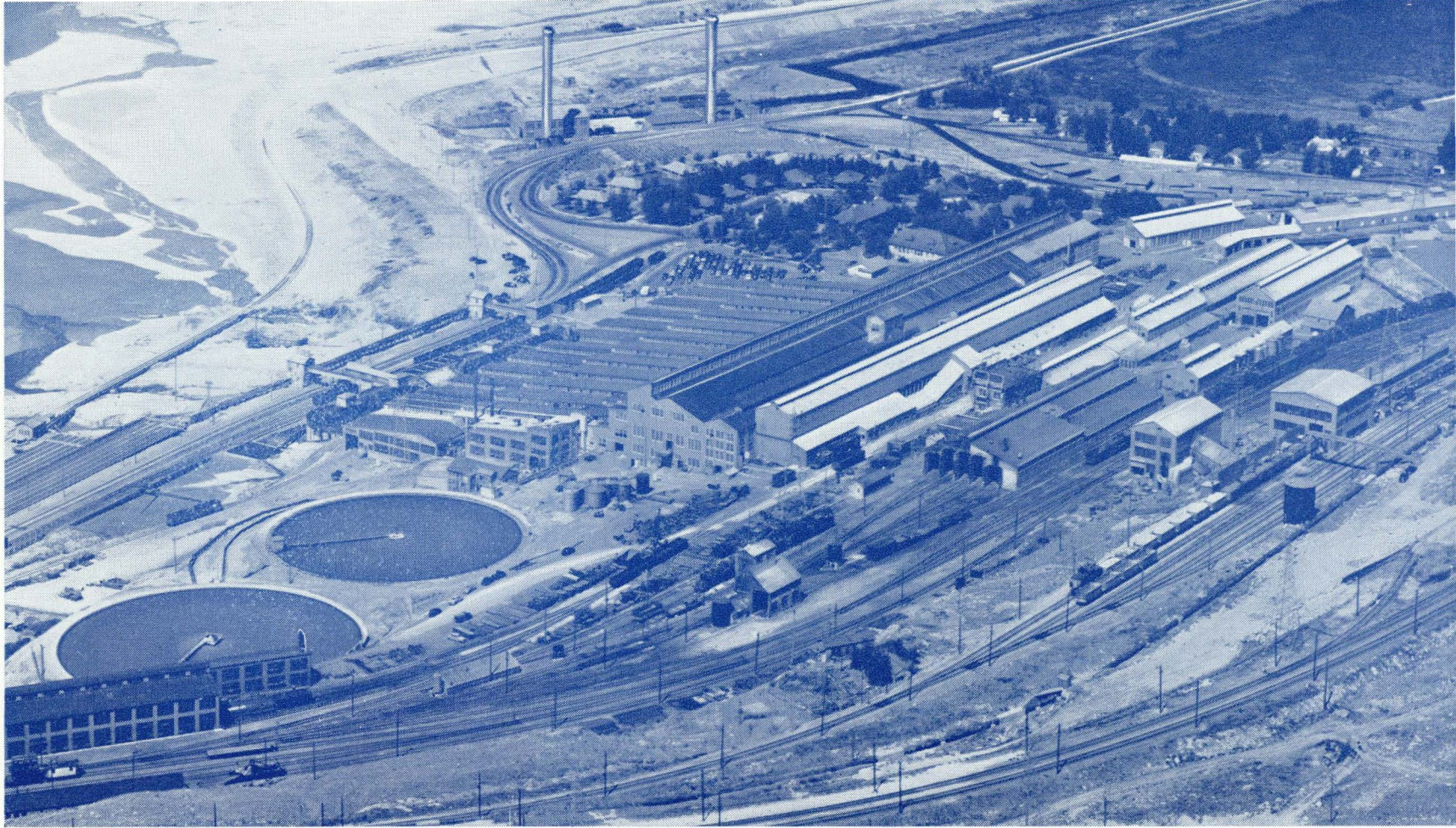
A recent picture of the same mill. In the left background is part of the 6,000-acre tailings pond which receives the waste material after the ore has been milled. Circles in left foreground are thickener tanks for flotation feed.
