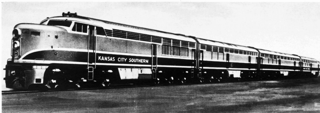
Fairbanks-Morse four-unit 8,000 h.p. freight locomotive for the Kansas City Southern, used in 1947 but subsequently divided into two double-unit 4,000 h.p. locomotives
