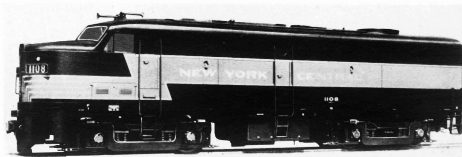
Alco 1,580 b.h.p. Bo-Bo unit for freight service on the N.Y.C., 1946-47; as a rule two to four units of this power were coupled together
