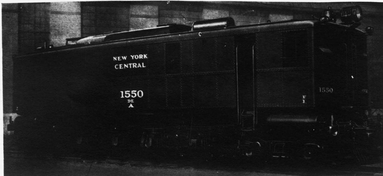
Early effort of the New York Central at a line-service locomotive, a 2-Do-2 diesel-electric of 750,800 b.h.p. and 130 tons weight, 1929
