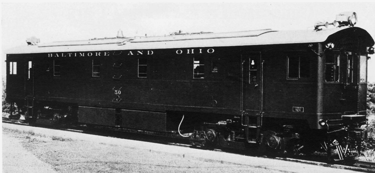
One of the first five Electro-Motive 1,800 b.h.p. main-line locomotives, all built in 1935, which was retired to St. Louis museum in 1959 after being in service on the B. & O.
