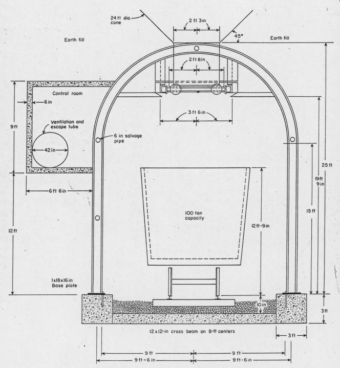
Section of loading chute inside tunnel shows control room, vent tube, loading gate and other details.
