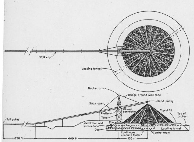
General arrangement of Sunnyside's high-capacity unit-train loading facility details major features, including the conveyorway, tunnel, steel cones, loading gates and tower. More than 400 tons of steel was used.
