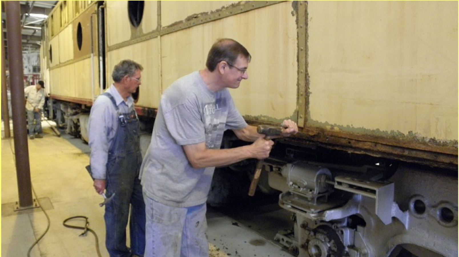
Here Tim Johnson and John Bateson show how to remove rusted old channel.
