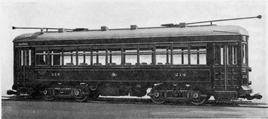
SEMI-CONVERTIBLE CARS FOR EASTON. All-steel car, including steel roof, for high-speed service on the Bethlehem Division of the Easton Transit lines. Mounted on Brill 27-M.C.B.1 Trucks
