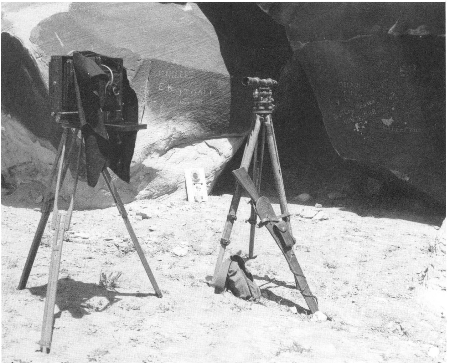
On June 7, 1981, a century to the day after E. Miller and J.T. Daly paused to carve their names in sandstone, Jim Ozment assembled this arrangement of surveyor's paraphernalia in front of "Inscription Rock," in the desert south of Cedar Mountain, Utah. A cumbersome 6-1/2 by 8-1/2-inch glass plate view camera (representative of the times), a surveyor's transit, level, carbine rifle and knapsack tell a silent but eloquent story of what it was like to find a path through the wilderness for a narrow gauge railroad. John H. Averett and H. A. Petty left their names a day earlier, June 6, 1881. The reader can decide at what point in time graffiti becomes an historic inscription.
