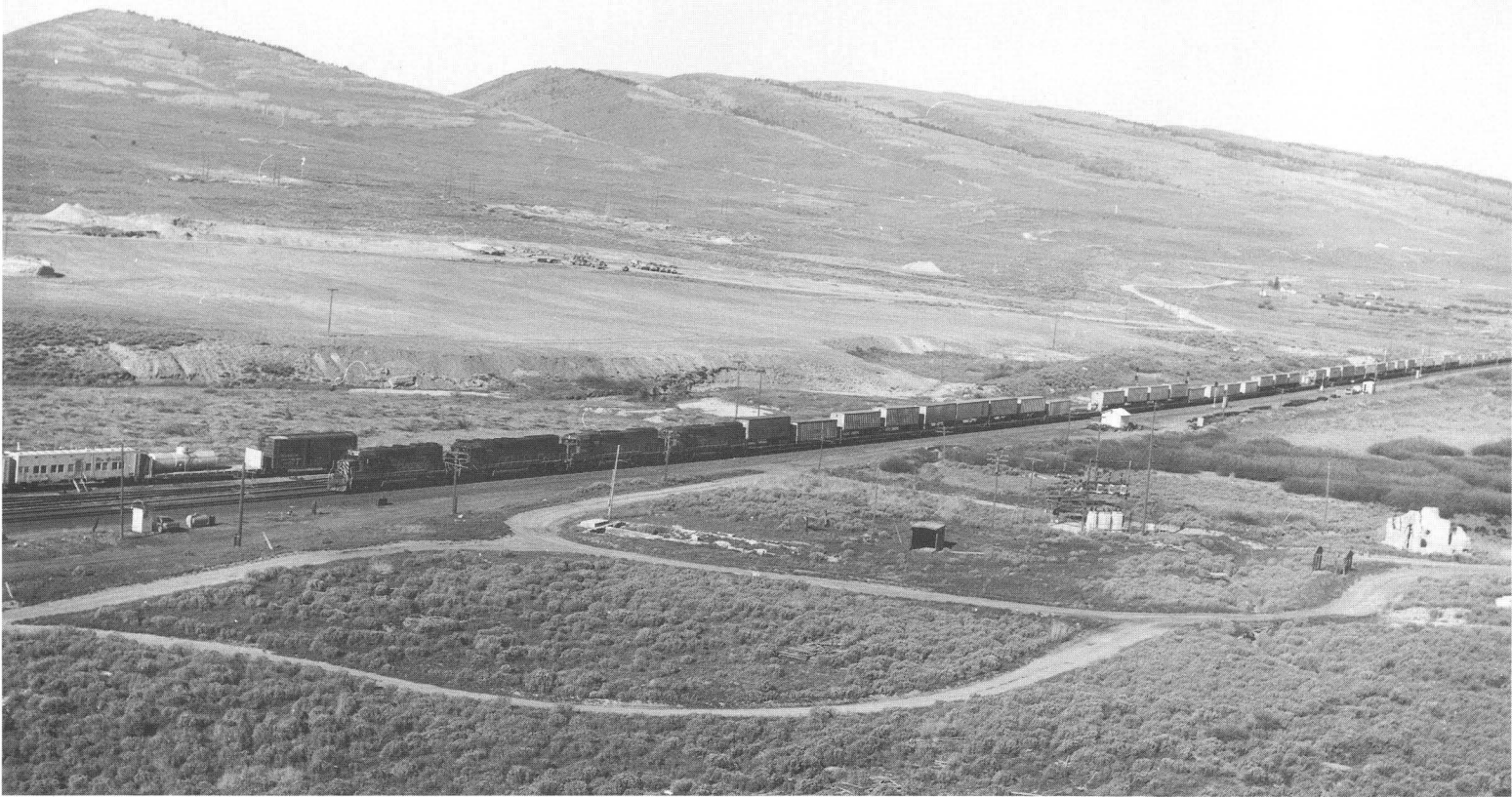
Only a few foundations mark the spot of the town of Pleasant Valley Junction (later, Colton). An eastbound D&RGW piggyback train is running on the westbound main, a feat accomplished safely by having Centralized Traffic Control signalling on the entire mainline between Denver and Ogden. Some outfit cars are spotted in the old Colton yard, October 17, 1983. (J.L. Ozment photo) (below) Shortly after the roundhouse view on the opposite page was taken, Ercanbract and Fireman "Shorty" Moran moved the 272 onto the turntable. Beyond the flatroof coach in the background can be seen four-wheel Denver & Rio Grande cabooses 74, identical to No. 49 now restored and exhibited at the Colorado Railroad Museum. (Junius Young photo, Fred W. Voll collection)
