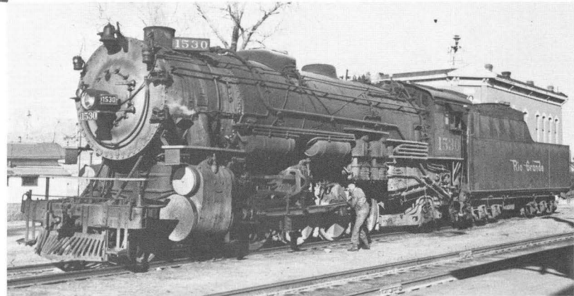
(Right) The engineer of M-67 class 4-8-2 No. 1530 tinkers with his engine's left side rod assembly as he awaits a call for helper service at Buena Vista, Colorado, in February 1941. (John W. Maxwell) Old man winter applied a streamlined casing to the boiler of No. 483 at Cumbres Pass, in a gesture probably not appreciated by the crew. (Robert W. Richardson)
