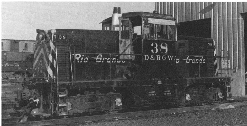
No. 38 was the last of the six 44-ton GE units to survive on the roster. It is shown outside the diesel shop at Burnham in the summer of 1964. (Ed Fulcomer)
