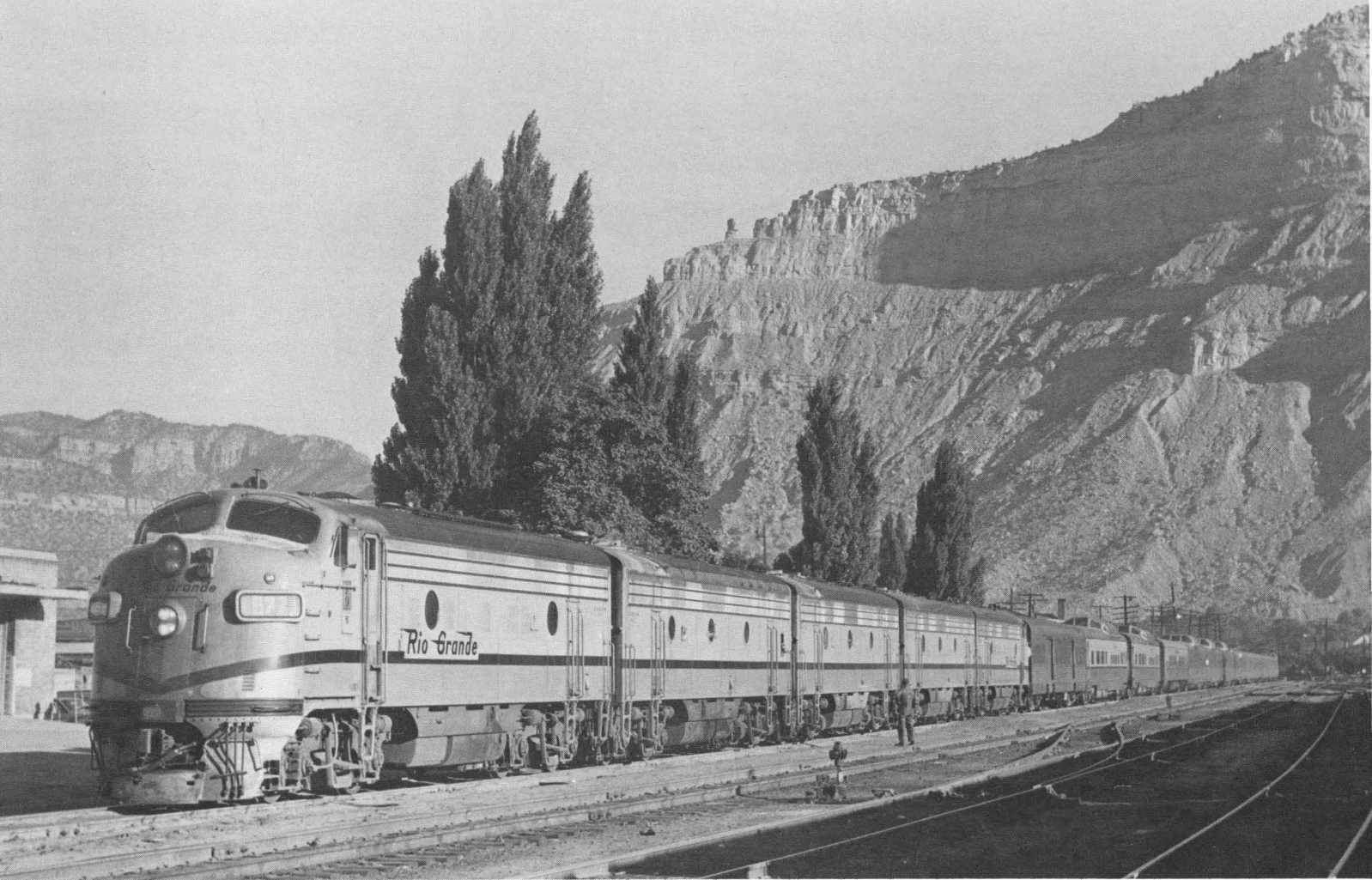
F9A 5771, destined to become famous as the D&RGW's last "covered wagon" A-unit, leads four mates into Helper, Utah, on September 15, 1968, with the eastbound California Zephyr. Three extra cars have put all 8250 HP to good use over Soldier Summit. (Ed Fulcomer)
