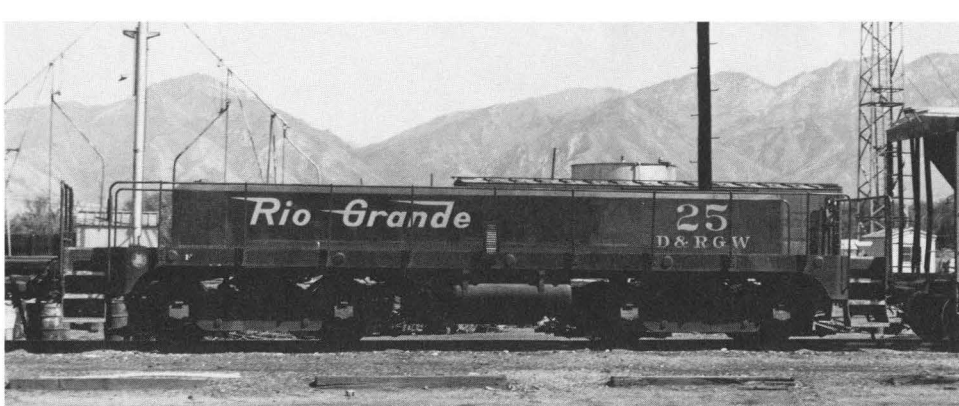
Scale test car 25 at Salt Lake City in 1972 had started life as Baldwin V0660 switcher 68 before being converted to auxiliary booster 25 for service on the hump at East Yard, Grand Junction. (Ed Fulcomer)
