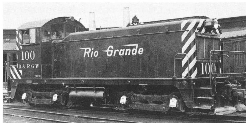
No. 7000 works Pueblo Union Depot less than a month after its delivery in early 1941 (Richard H. Kindig-Ed Fulcomer Collection). Soon renumbered 100, it was still sub-numbered 7000 when the photo below right was taken. It also had received extended exhaust stacks and a cab bay window. (Michael Davis Collection)
