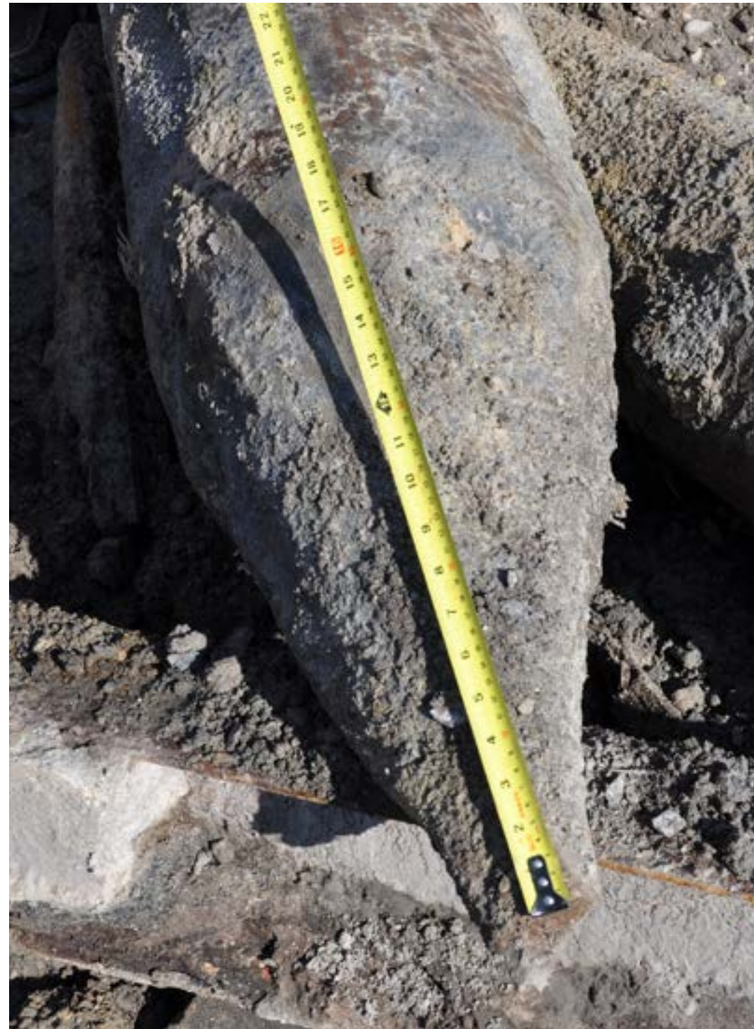
Figure 14. Example of incomplete wood friction pile point.
