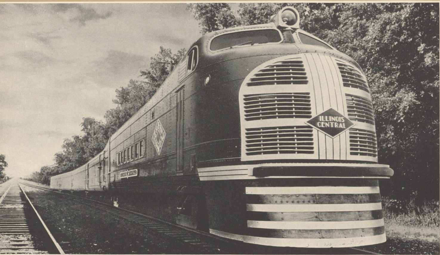
The GREEN DIAMOND, powered by a 16-201A GM Diesel Engine was one of the early streamlined trains.
