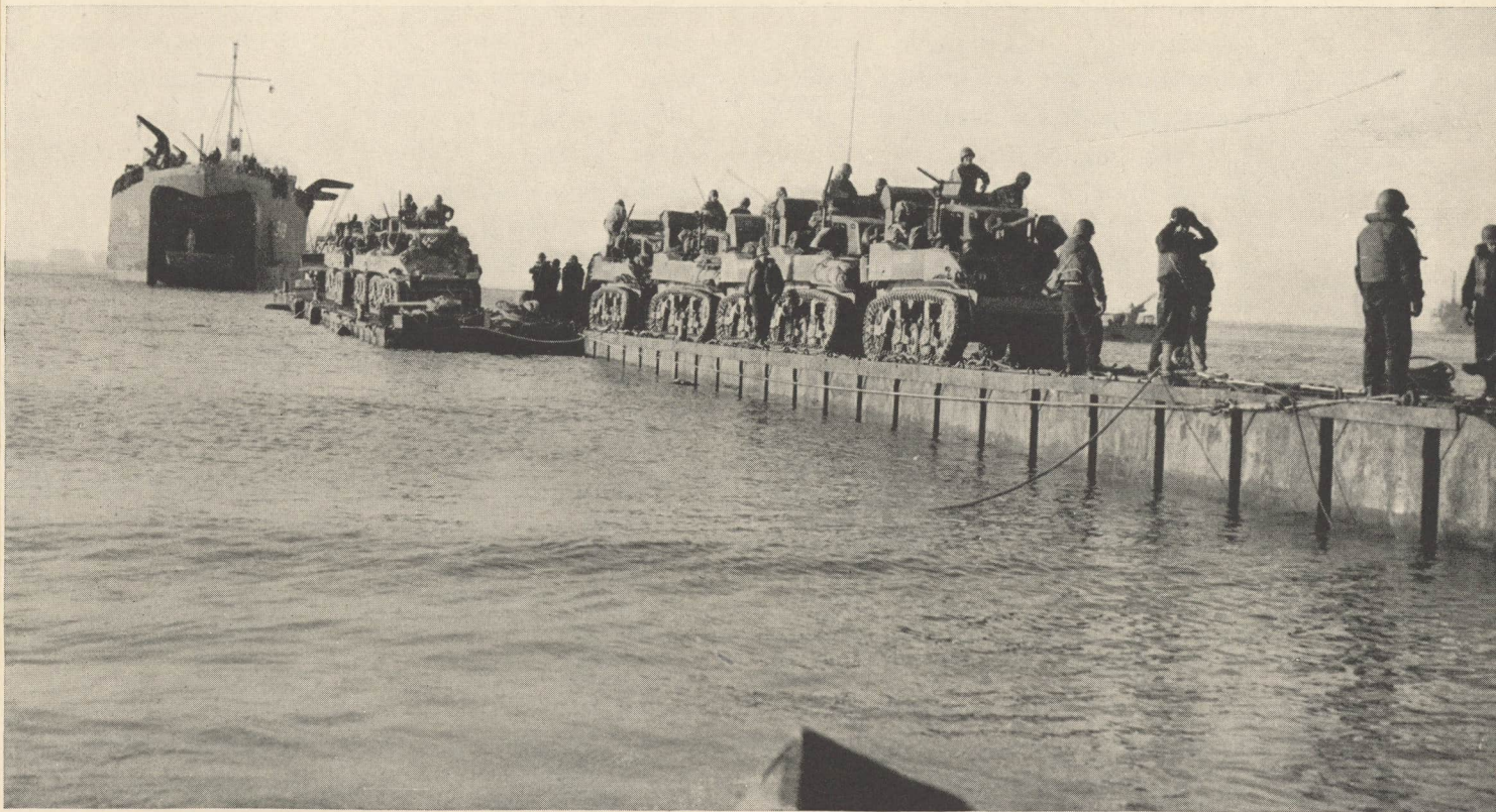
From this position on the side of the ship the LST can drop pontoon gear to establish a "road bed" for landing
