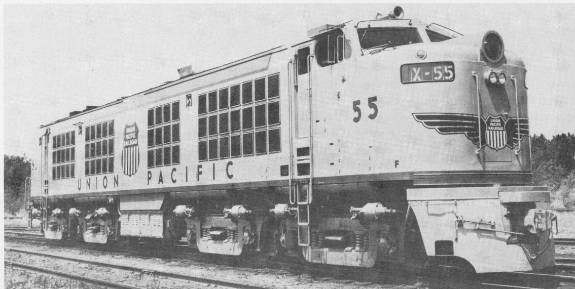
The first series of General Electric's gas turbine locomotives delivered to the UP had enclosed catwalks.
