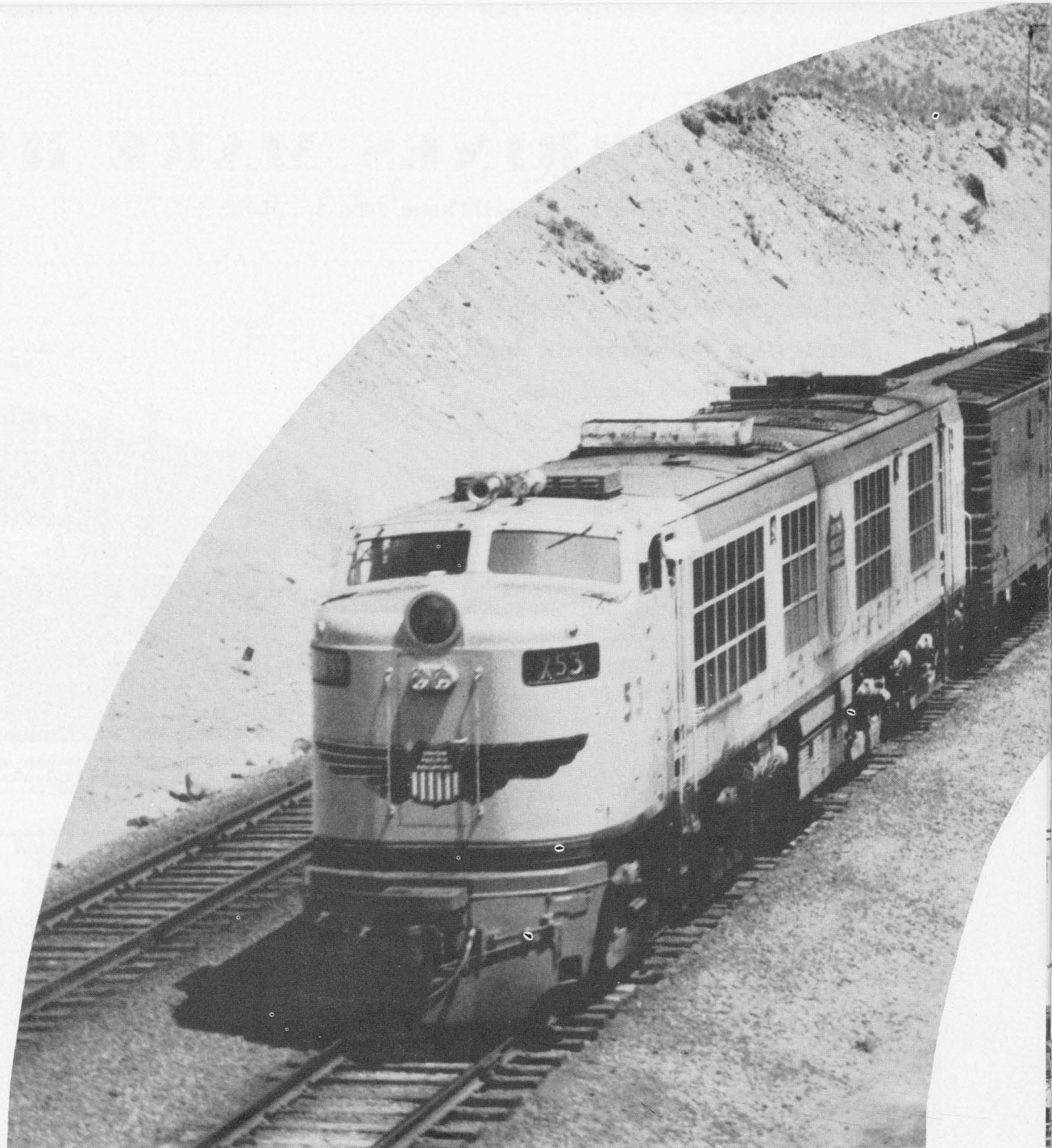
One of the original gas turbine locomotives delivered to Union Pacific is shown pulling a heavy freight train through Wasatch Canyon.
