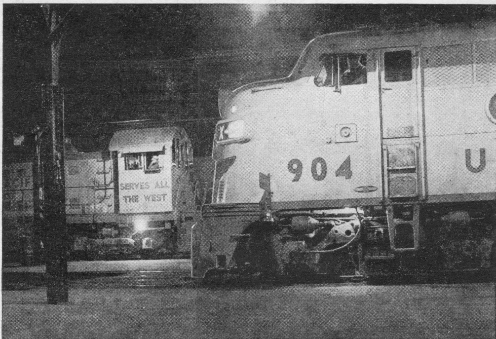
BLUE FLAG hangs on cab side of UP diesel No. 904, indicating that inspection and servicing crews are still at work. In the background a switcher awaits its next assignment. Diesel goats are used at Ogden Union Station to pull in and pull out certain trains
