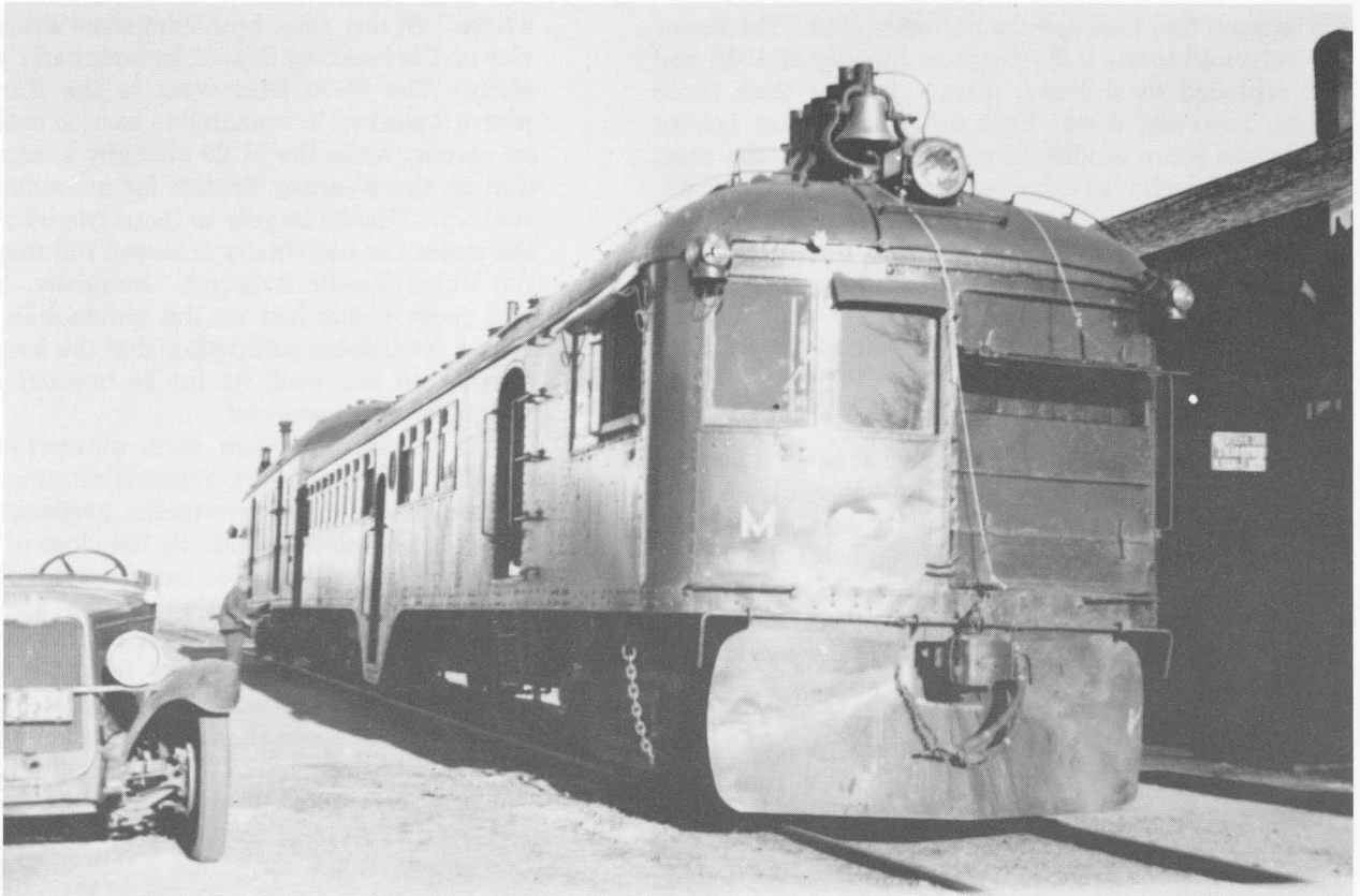
The M-29, with Railway Post Office car in tow, had already donned a pilot plow for winter operation when viewed as Train 518 at Callaway on an autumn morning in 1946. The slightly battered nose probably resulted from a previous altercation with a highway vehicle at a grade crossing. The Model A Ford at left, previously modified into a homemade pickup, conveyed the U.S. mail between the trains and the Callaway post office.
