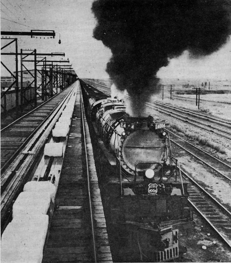
FRESH PRODUCE in a block of reefers in Extra 4004 East pulls into the machine icing dock at Laramie, Wyo., beside a belt of 300-pound blocks of ice.
