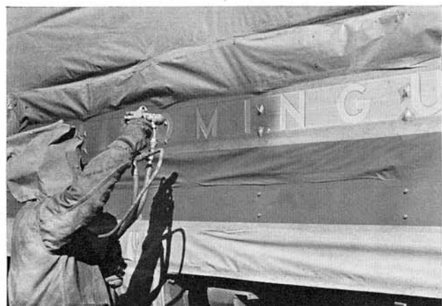
Spray painting the lettered area in red. The Tape serves as a stencil for the lettering, and as protective masking of the previously-applied yellow.
