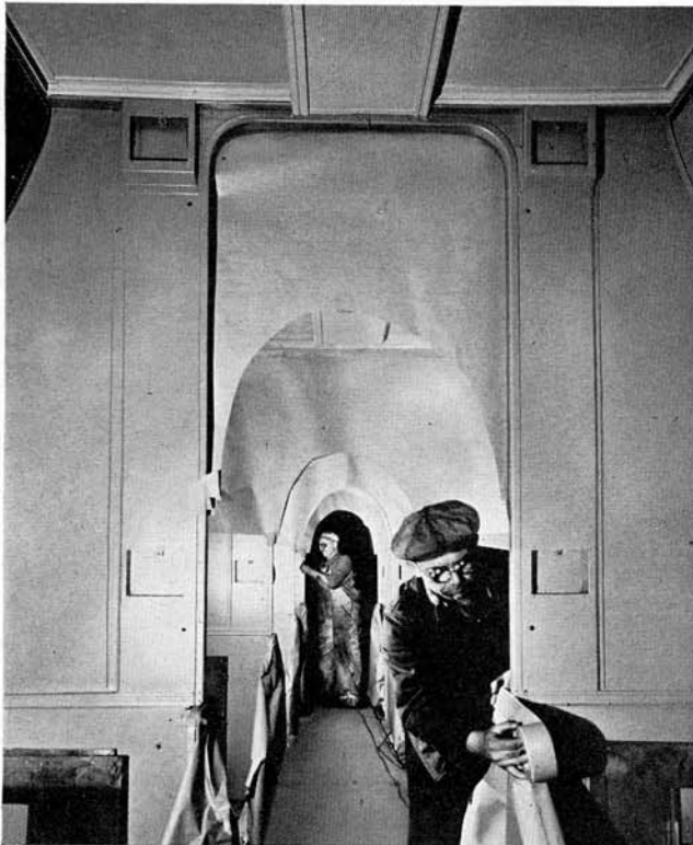
Preparation for spray painting. All surfaces that are not to be painted in the next operation are masked off with kraft paper held securely in place by Paper Masking Tape.
