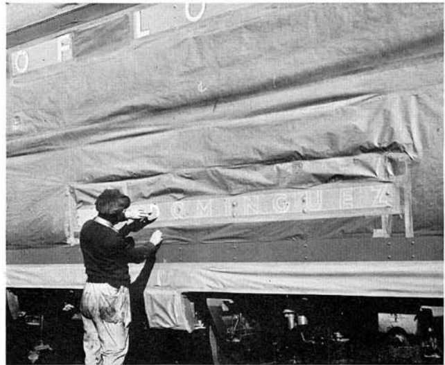
Cutting out letters for removal from a strip of Masking Tape that will serve as a stencil for spray painting the name of the car. The Tape that remains masks off the yellow surrounding the lettering.
