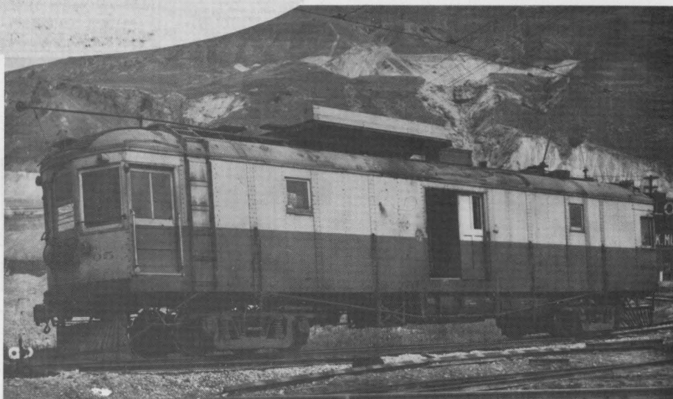
Car 01 (above) weighed about 40,000 lbs. and had two GE 205B motors and Baldwin 78-30 trucks, 36" wheels. Its body lines suggest the possibility that it might have been a steam coach before electrification of the SL&O. Photo by JS in 1942.
