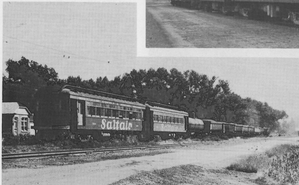
Open trailers 301-313 were 55'8" long, seated 100 and weighed 20 tons. (FF)
