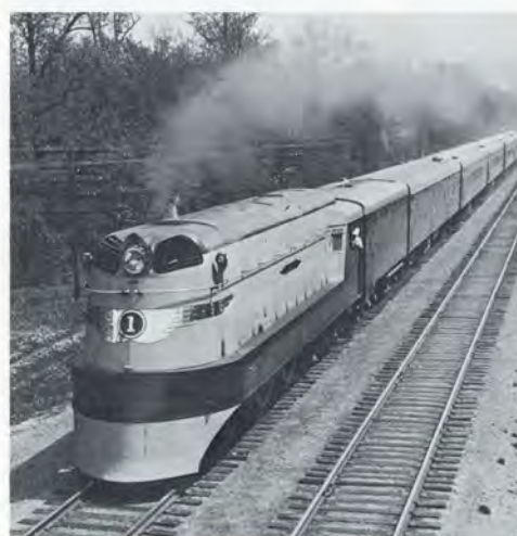
No. 1, the original 1935 Hiawatha, was the first newly-built streamliner. Class "A" 4-4-4 "Atlantic" burned oil, had top speed of 120, had 84" drivers and 88' overall length.
