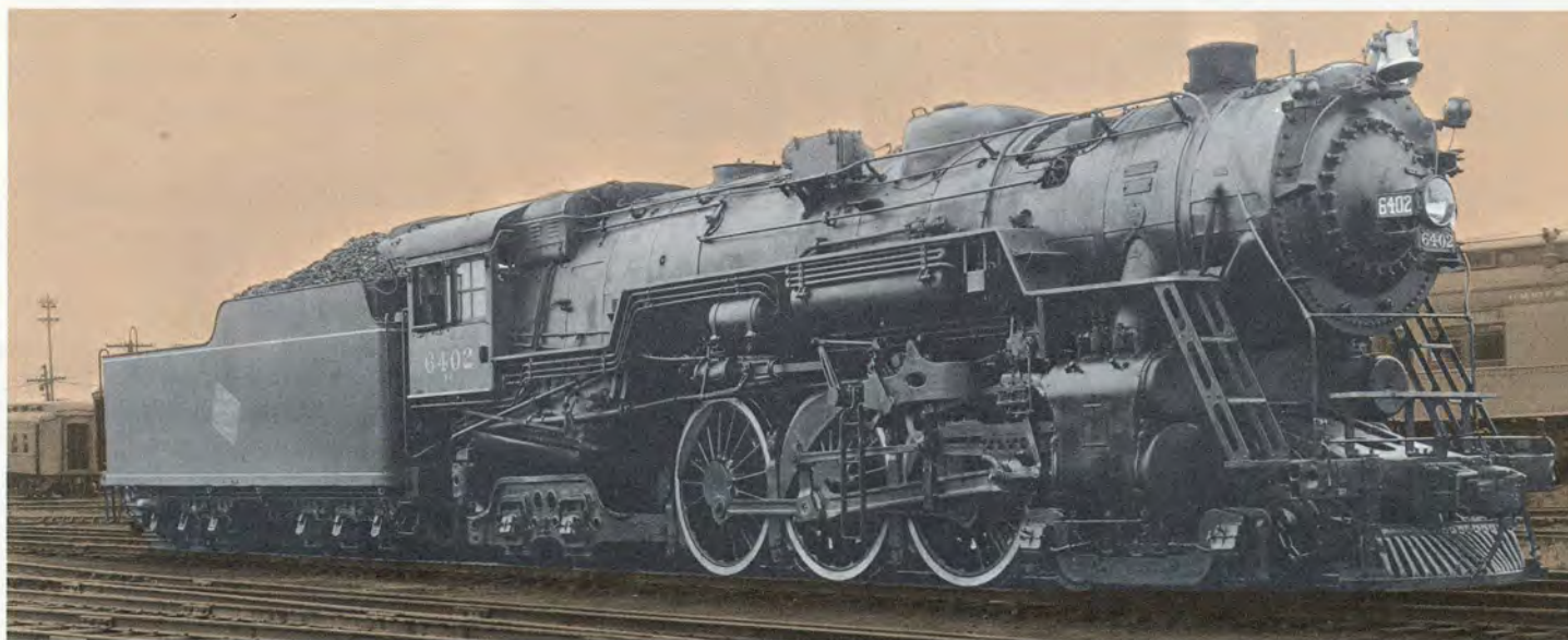
▼ No. 100 was an F7, 4-6-4 built in 1938 for a Hiawatha introduced that year, with newly designed passenger cars.
