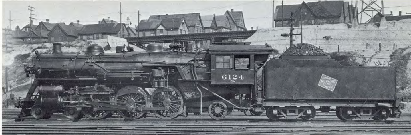
▲ No. 6124 and other F3 "Pacific locomotives were real workhorses over the years, combining speed with hauling power.
