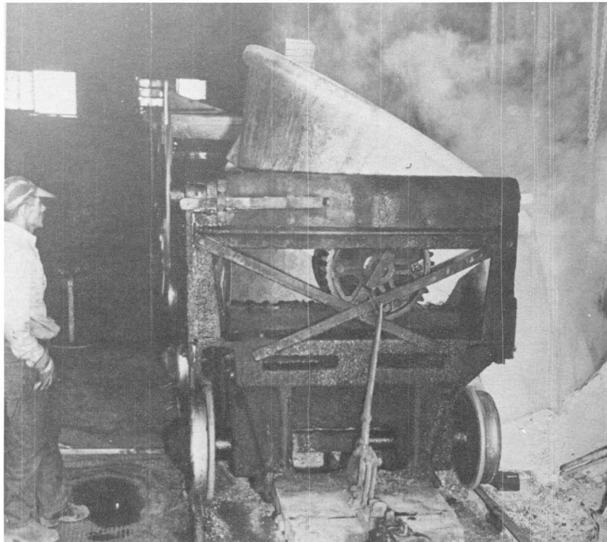
Pouring molten slag to slag furnace. Slag from the blast furnace is treated to recover lead and zinc.
