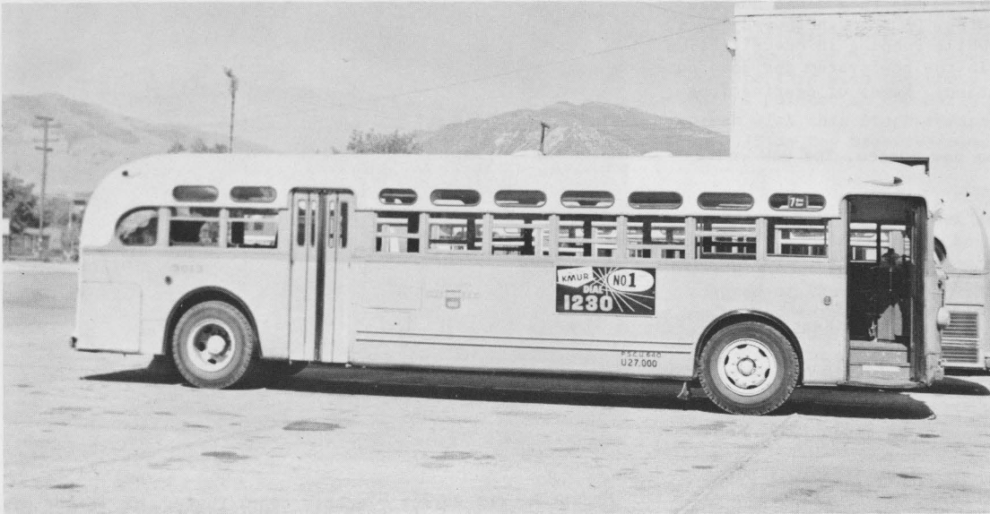
One of SLCL's original TG-4007 buses, 3013 had been repainted from the orange and cream scheme to the orange, green and white, and rebuilt with a 6-71 diesel engine by the time this photo was taken in June 1959. The large black numbers of the PCL network have also been replaced with NCL's gold numbers.
