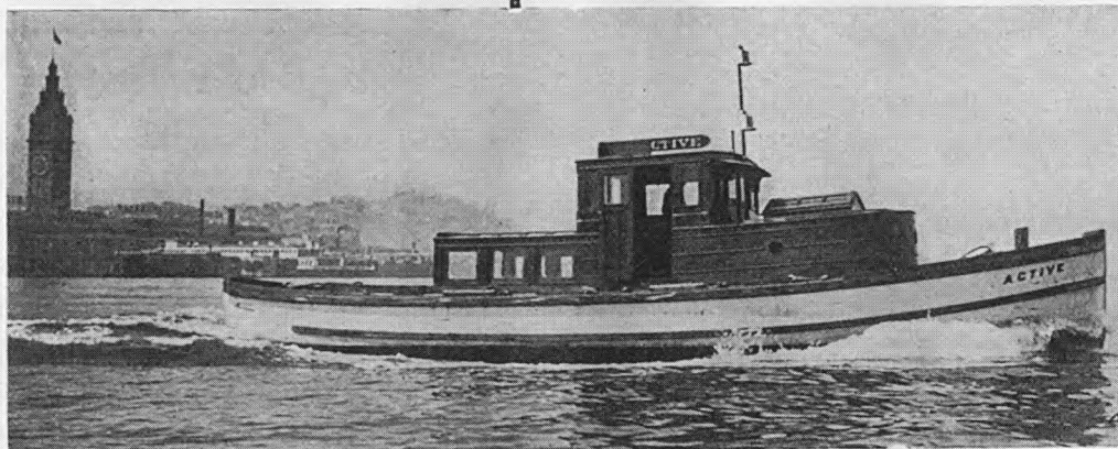
The "Active," Owned by the San Francisco Examiner. She is 50 ft. long and is Powered with a 50 h. p. CORLISS Engine
