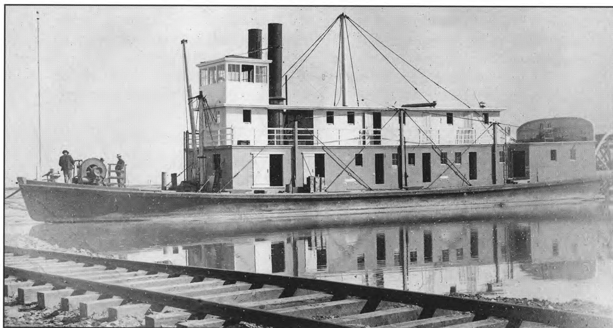
Finishing touches are added to the steamer after being completed in the water. According to the most reliable source (Oscar King Davis, 1906) the Promontory was 127 feet with a draft of only 18 inches. California State Railroad Museum, Collection: 387-253 No. 16979
