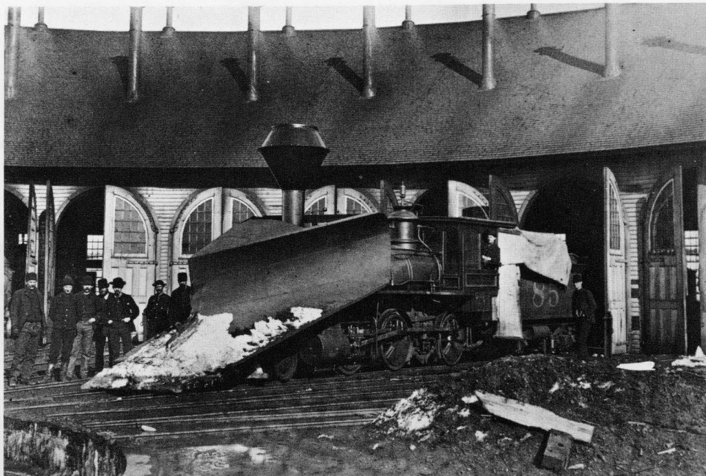
In the early days when drifts were big and engines were small, the wedge plows dwarfed the locomotives on which they were installed.
