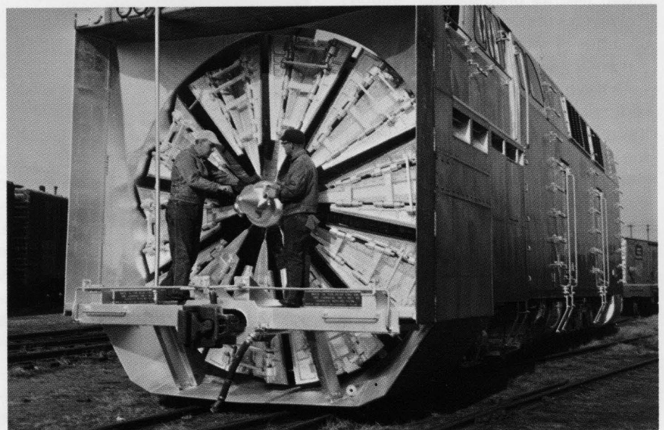
The 12-foot diameter of the rotary wheel on 900081 is apparent when compared to the height of the men working on the blades.
