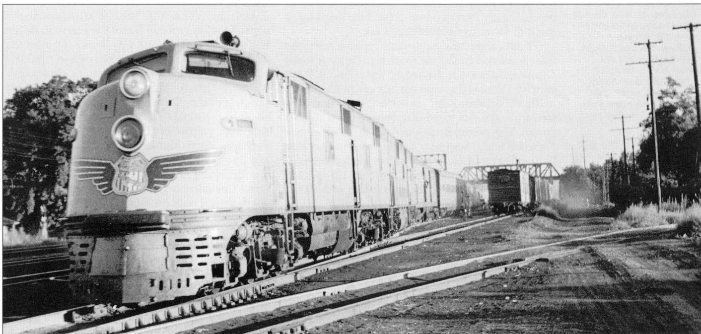
The westbound City of Los Angeles (Train 103) enters Ogden after passing beneath the Bamberger bridge in the distance. Leading the train is Union Pacific's GM-EMD E6A number 954A, built in 1940 as number 7-M-2A. This unit was retired in 1956 as number 993. This train will continue into Ogden Union Station. Upon departure it will be pulled back by an OUR&D switcher to approximately its current location and will depart bound for Salt Lake City, Las Vegas, and Los Angeles via the 30th Street wye under its own power. In the immediate foreground is the connection for the passenger balloon track, which allowed OSL trains to enter Union Station via the same direct route as UP trains. (Emil Albrecht, James W. Watson Collection)
