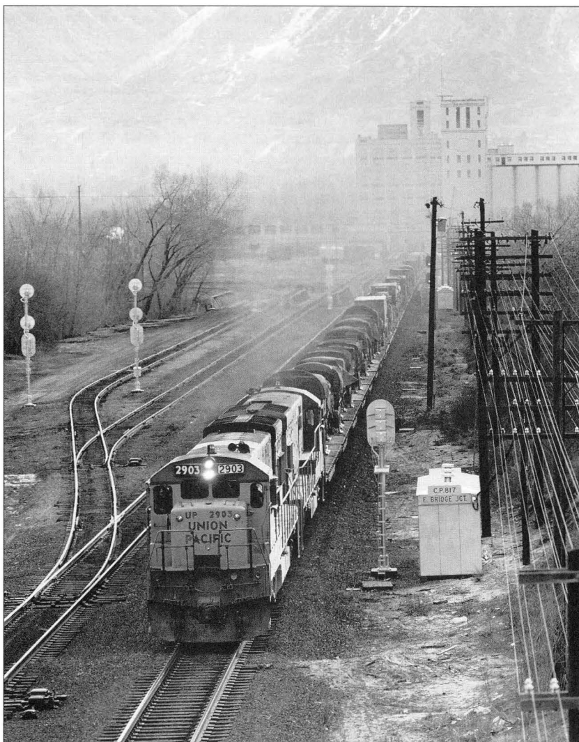
Bridge Junction was the connection between Ogden Union Railway & Depot Co. and Union Pacific's Oregon Short Line from Salt Lake City. The junction came into being with the completion of the Sand Ridge Cut Off in 1906, and was double-tracked in 1912. In 1928 the Shasta Track (far left in this view), with its two adjacent home signals, was added as a run-around track for OSL trains between Salt Lake City and Idaho. Here we see Union Pacific U30C number 2903 at East Bridge Junction (Control Point 817, situated 817 miles from Los Angeles) in August 1982, leading a special military train bound from Kansas for training exercises in southern California. (D. B. Harrop)
