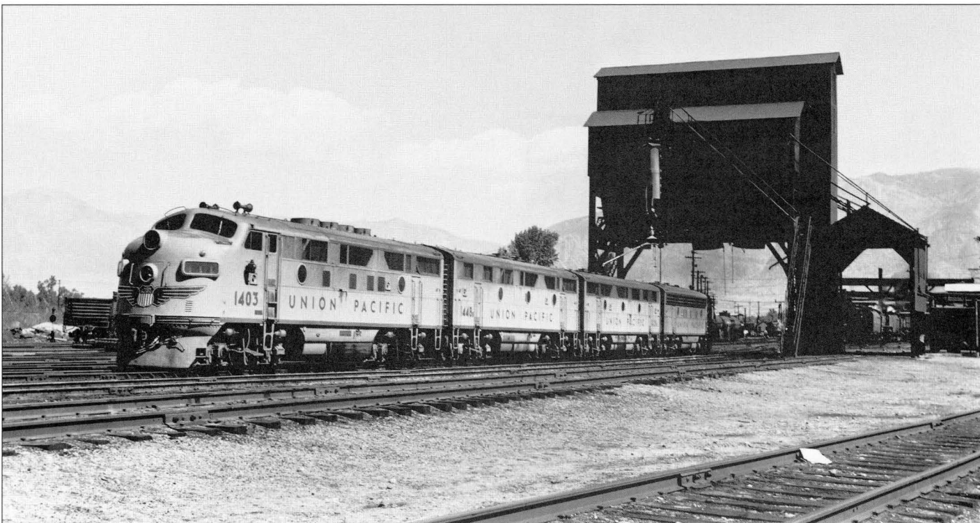
Union Pacific dieselized the west end of its railroad from 1947 to 1952 with a large fleet of 237 cab units from General Motors' Electro-Motive Division, and in 1947 and 1948 with 88 cab units from American Locomotive Company. Both types of units regularly ran into Ogden, from both Idaho and from California. Here, EMD F3 1403 and three stablemates await their next assignment under Union Pacific's large coal chute at Ogden. (Emil Albrecht, James W. Watson Collection)
