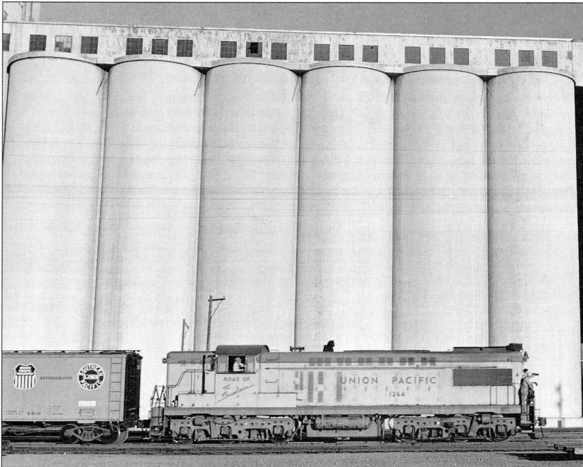
The Baldwin-Lima-Hamilton Corp. (Baldwin Locomotive Works until 1950) built 168 examples of its 1,600-horsepower AS-616 model road switchers between 1950 and 1954, of which Union Pacific purchased only six. Southern Pacific purchased 56 units, using them as road switchers, the assignment intended by Baldwin. But UP needed heavy switchers for its new hump yards in Pocatello and North Platte, and for heavy switching at Ogden. Two of UP's six units were immediately assigned to Ogden upon their delivery in late 1951, and both units (numbers 1264 and 1265) remained at Ogden throughout their 17-year careers. A regular assignment called for them to pull entire trains between the two OUR&D yards, the main yard between 20th Street and 29th Street, and Riverdale Yard between 31st Street and Riverdale Road, passing the large Sperry mill at 30th Street, shown here as UP 1264 heads toward Riverdale with a cut of interchange traffic between SP and UP. (Emil Albrecht, James W. Watson Collection)
