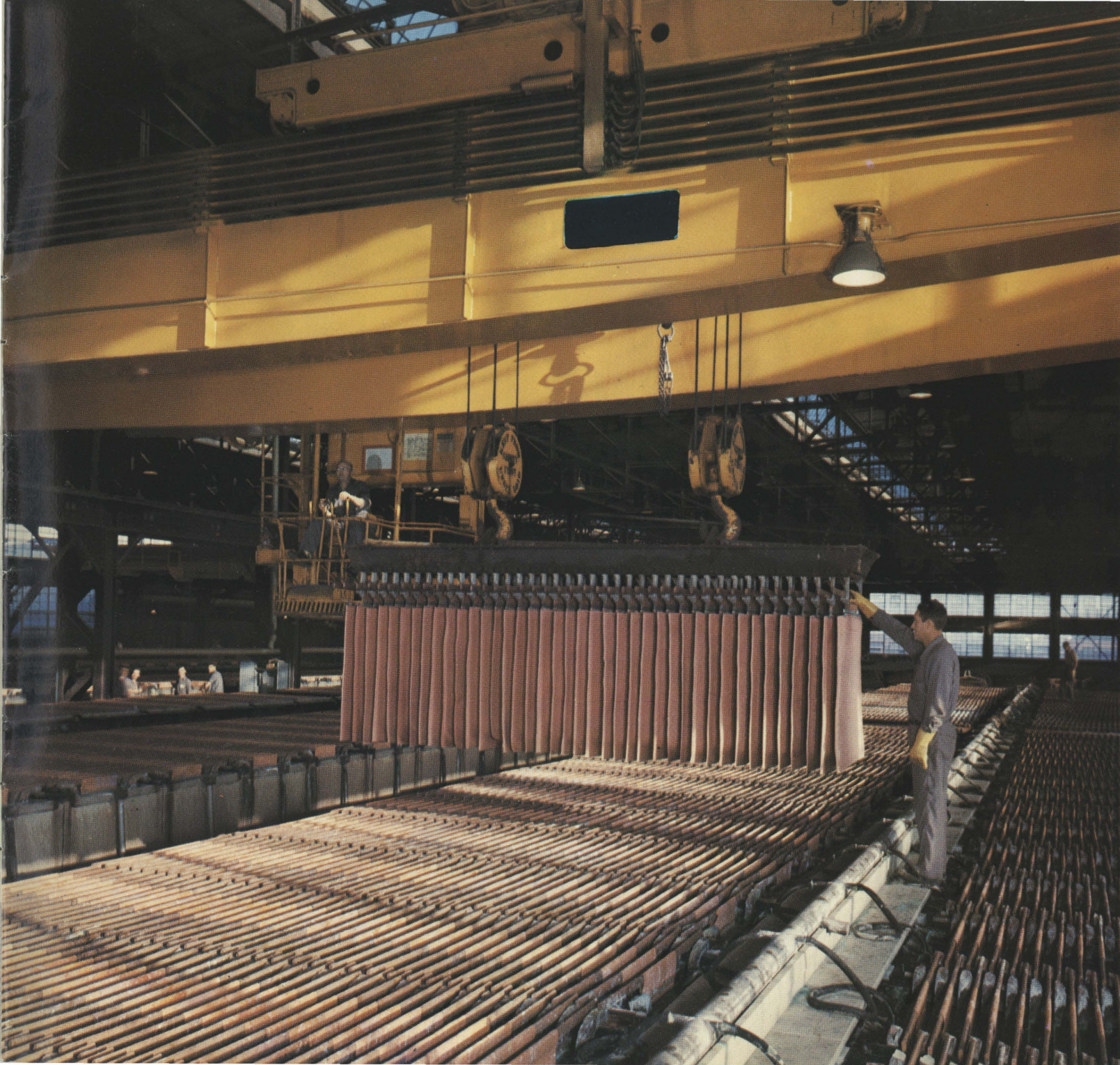
Copper cathodes being lifted from electrolytic cells at Kennecott's Utah Refinery. After cleaning, the cathodes are melted and cast into salable shapes.
