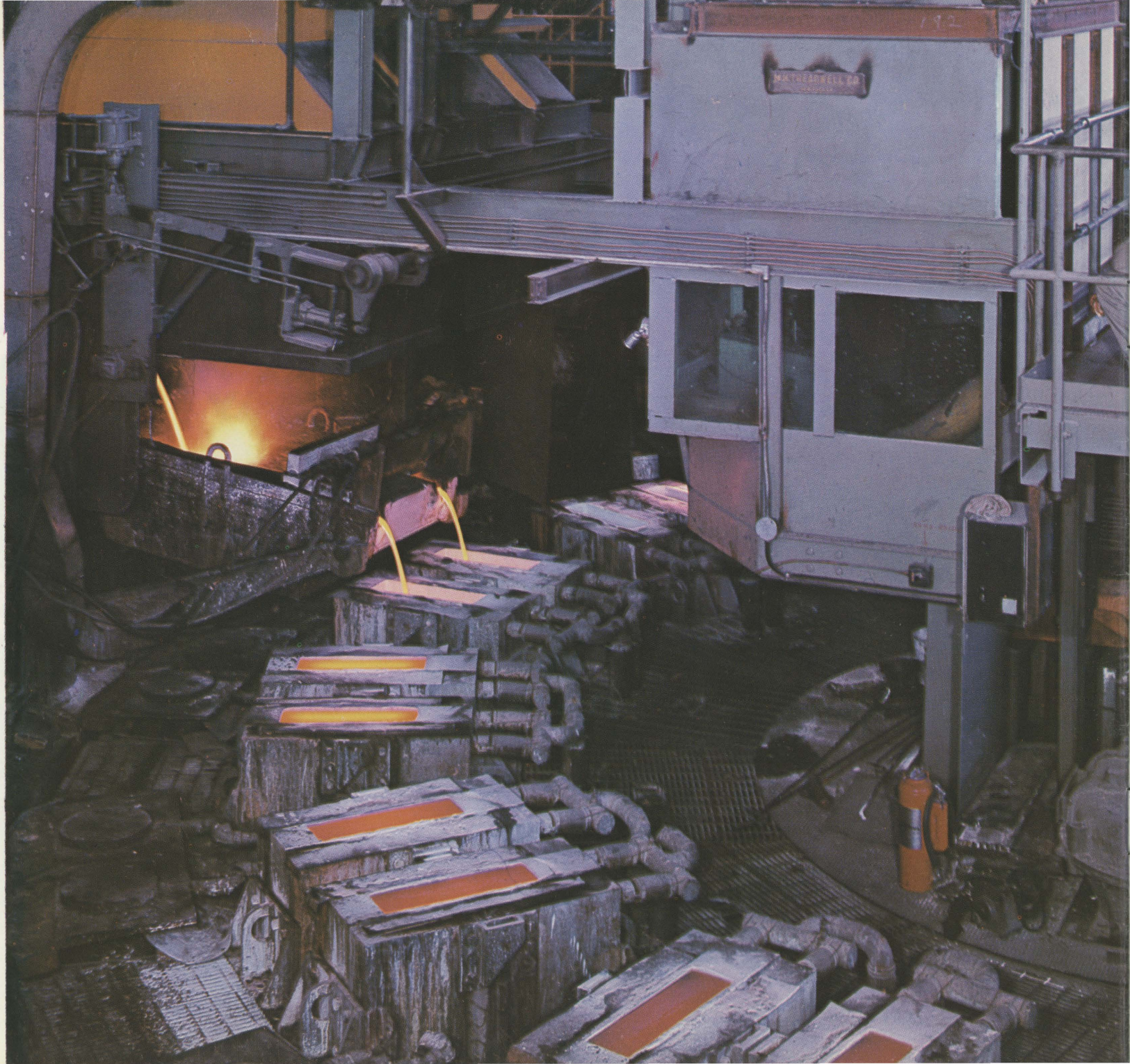
Casting copper into cakes makes a brilliantly colorful display at Kennecott's Utah Refinery.
