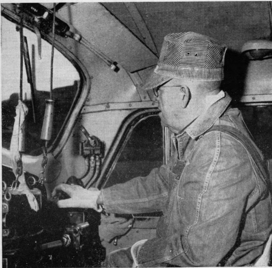
Santongue has his hand on the electric brake valve, ready to make an application to reduce speed on a curve outside of Los Angeles. This is the cab of the City of Los Angeles on a different day; the diesel is the 985, which has a slightly different arrangement of its controls.
