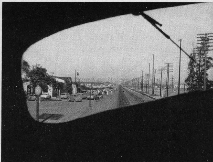
First stop out of Los Angeles is the station at suburban East Los Angeles. This is the way it looks to you from the fireman's seat in the cab of the diesel. You're running in C.T.C. territory, and the dispatcher has you on the left-hand track. The double track ends at Montebello.
