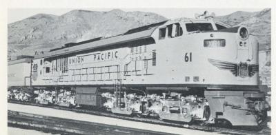
The new gas turbine-electric now on order by Union Pacific is rated 8500-hp, will develop a continuous tractive effort of 145,000 lbs. It's believed to be the most powerful internally-powered unit ever built.
