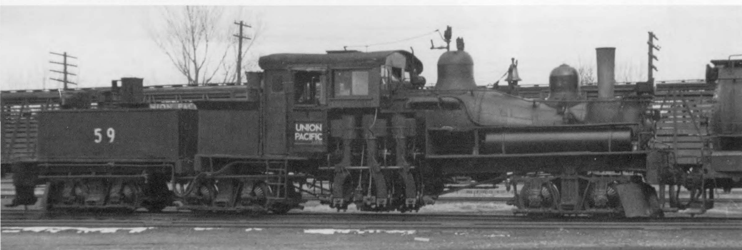
Another view of LA&SL 59 at Cache Junction. Note connecting rods are removed. - Emil Albrecht Photo, James L. Ehernberger Collection
