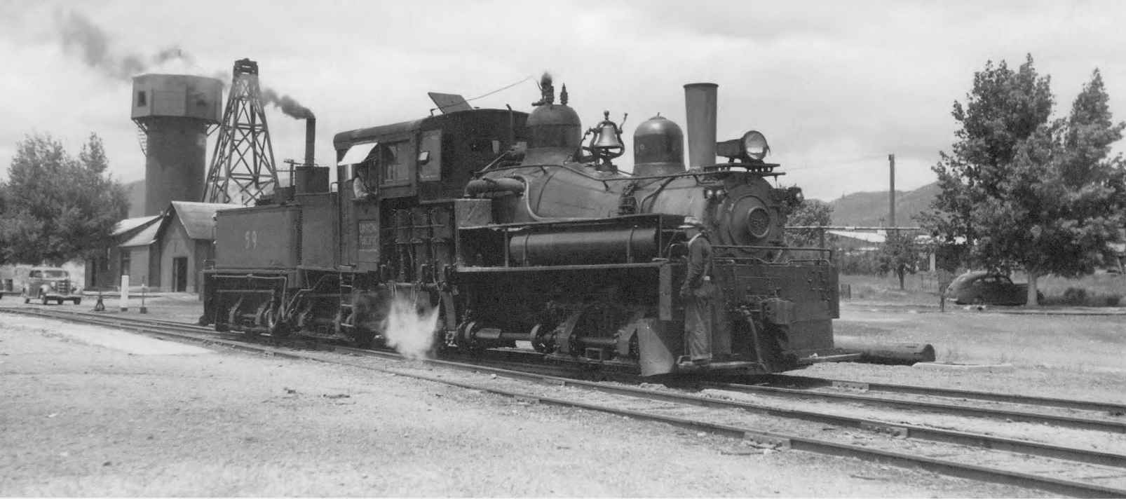
LA&SL 59 switching at Tintic on June 21, 1947. The LA&SL Shay locomotives assigned to the Tintic branches were oil fired. On a regular basis, oil arrived and had to be switched to the oil loading spur to fill the storage tank in the background. Another oil stand at Tintic also served to top off mainline trains. - Two photos, F. J. Peterson Photo, Donald Duke Collection
