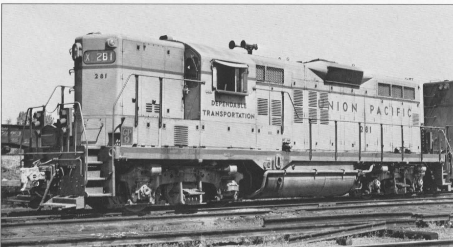
GP9 281 was the first EMD locomotive on UP to be turbocharged in the railroad's experimental program. The unit was completed in December 1955; however this view shows the unit as it appeared later in its life. The large fuel tank was applied in the 1960s, possibly when the AiResearch turbochargers were removed. Shown at Ogden, Utah, on May 29, 1965.
