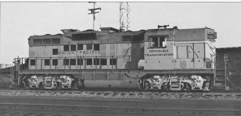
This view of AiResearch-equipped 261, taken in Council Bluffs in 1960, shows the rooftop air intakes and protective snow shields, along with the additional carbody openings that were cut to increase the volume of intake air available to the turbocharger. The rooftop air intakes were the final configuration of the AiResearch application, making the additional carbody openings an unneeded feature. The exhaust stacks on the AiResearch-equipped units were situated very close to where the stacks of a non-turbocharged GP9 were located. This view also shows the right-side features of the larger 2,400-gallon fuel tank for the heavy fuel modification.
