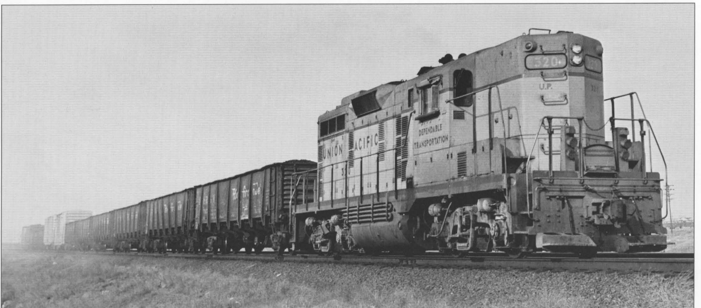
UP 320 as it appeared with the EMD turbocharger. This photo also shows the air cooling coils as they were after being moved because of the larger 2,400-gallon fuel tank. On an unmodified GP9, the cooling coils were mounted horizontally, under the walkways, not visible in typical photographs of standard GP9s. Cheyenne, Wyo., January 18, 1971.
