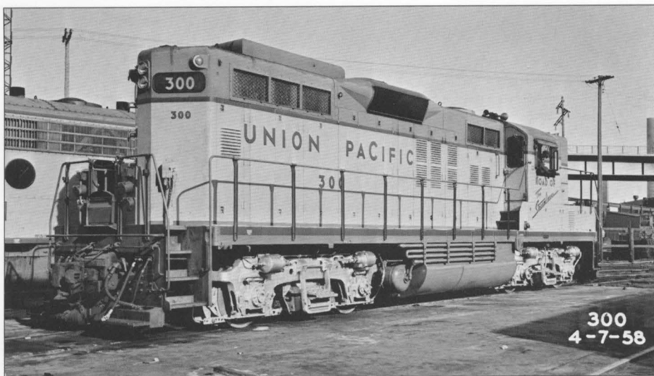
The heavy fuel modification was applied to UP 300 about a year before it was sent to EMD to have an EMD turbocharger installed. This view at Omaha in April 1958 shows the larger 2,400-gallon fuel tank used for the heavy fuel conversion. Note the air cooling coils mounted on the side of the larger fuel tank. On a regular GP9, these coils are mounted horizontally under the walkway. Also note the double set of louvers immediately behind the cab. Compare with the same area in the later view of turbocharged number 300.
