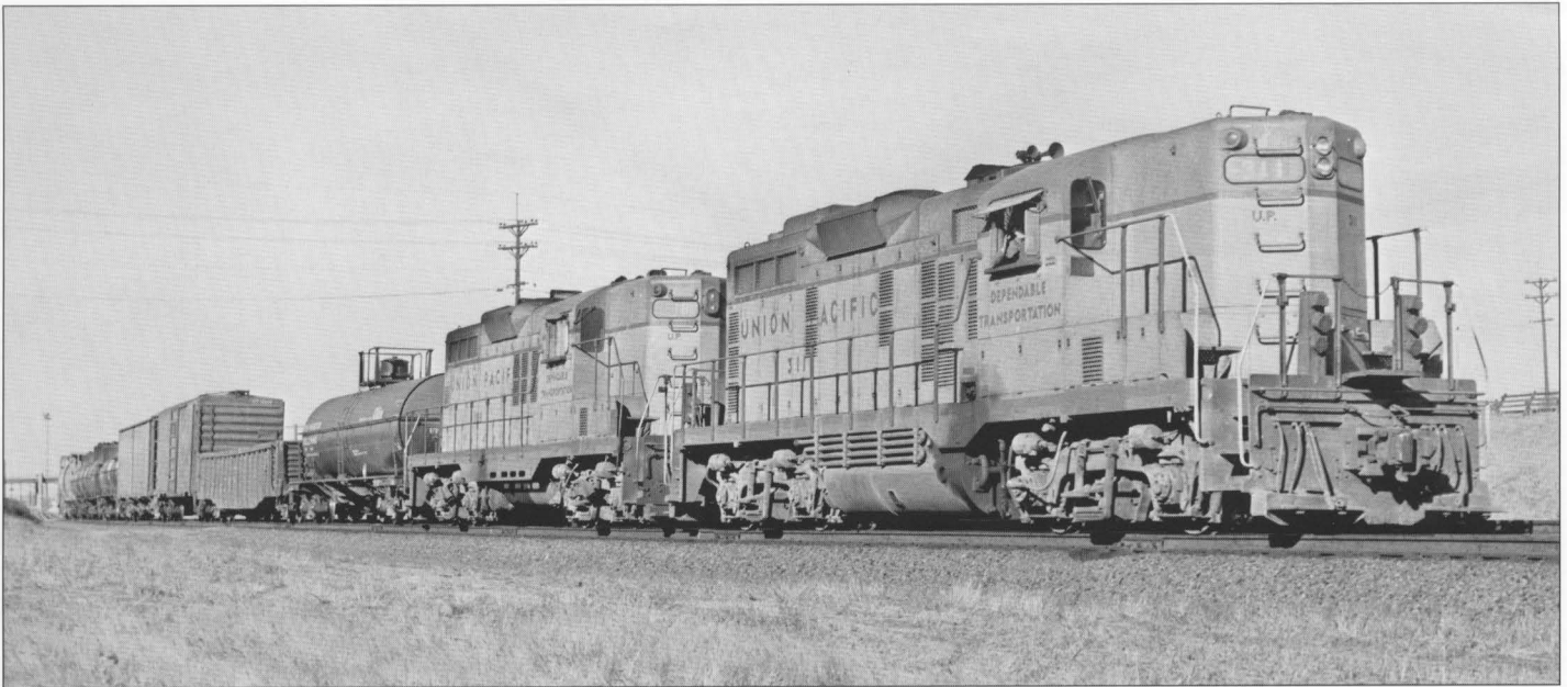
UP 311, shown with GP9 188 on an eastbound through Cheyenne, Wyo., on November 27, 1970, was one of six units that UP sent to La Grange in mid-1959 to have the EMD turbocharger applied. Visible on the trailing 188 is that unit's front exhaust stack, with UP-standard wire screen spark arrestor, which appears to be similar to the EMD turbocharger exhaust stack on the leading 311. This view also provides a comparison between hood-door louver patterns on the standard GP9 and the EMD-turbocharged GP9.
