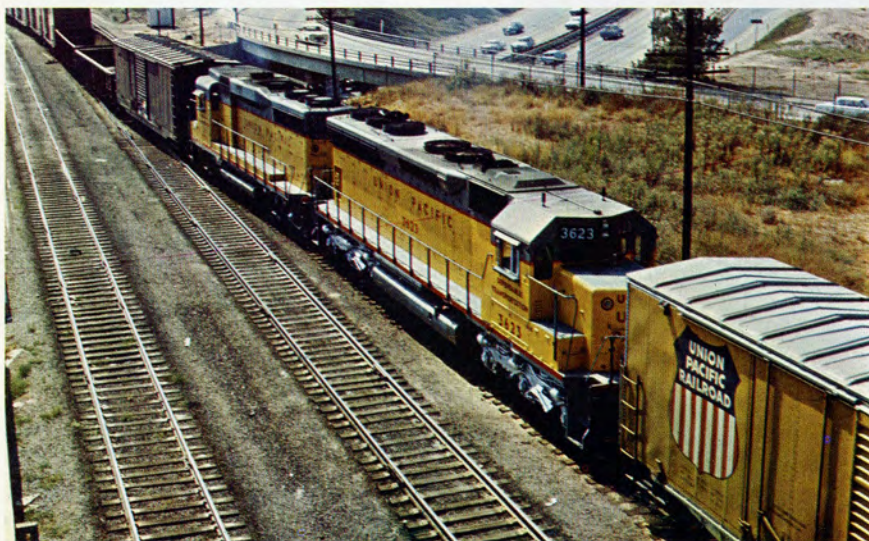
Mid-train robot locomotive . . . operated through control console in master unit. (shown above)
