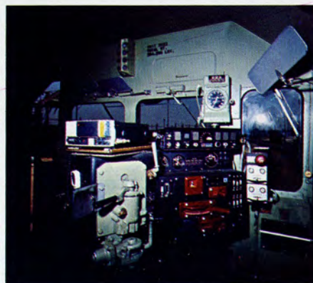
Mid-train robot locomotive . . . operated through control console in master unit. (shown above)
