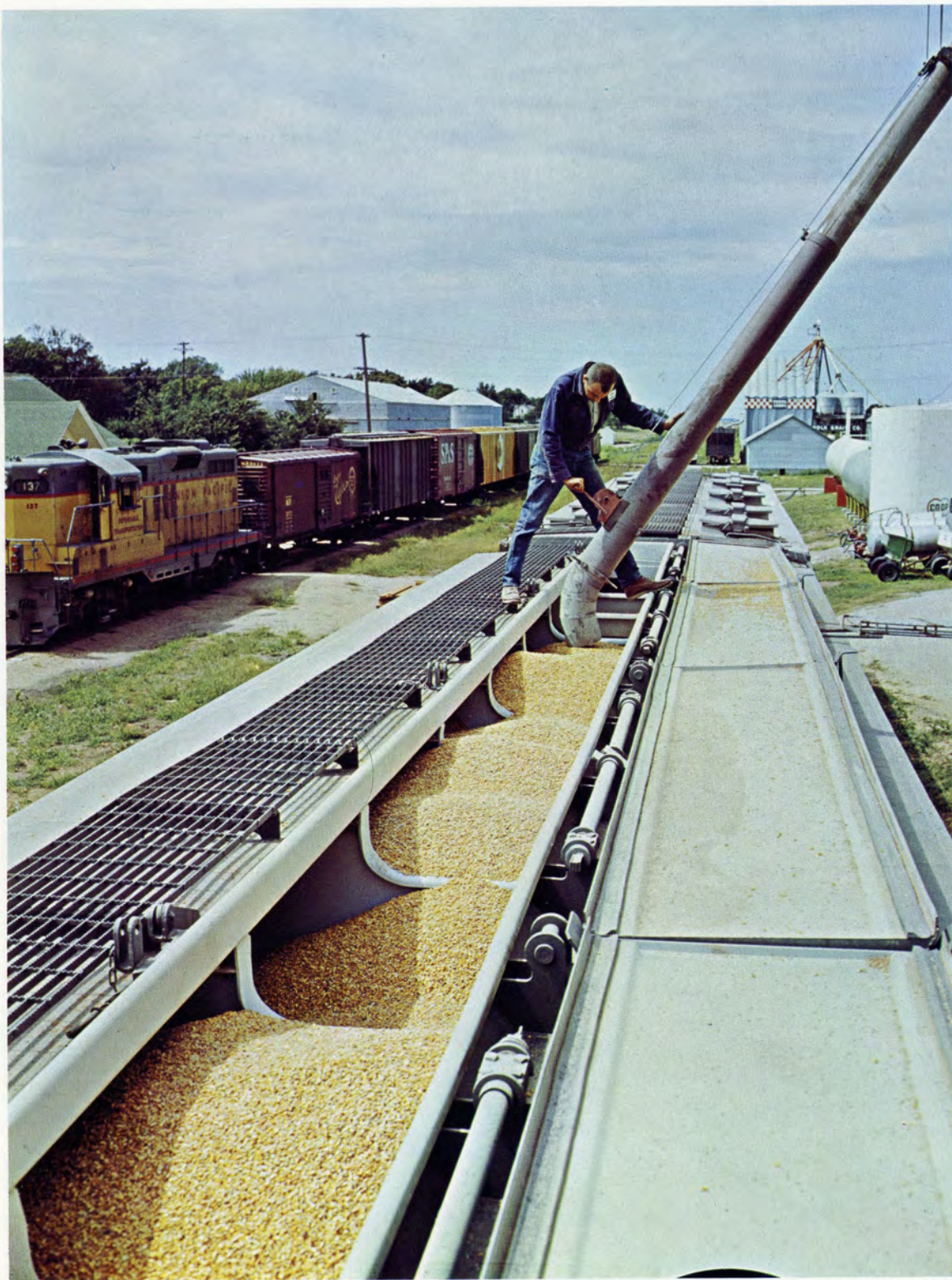
Air hose connection for unloading airslide hopper.
