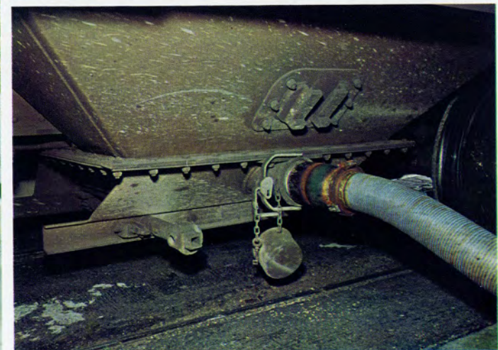
Air hose connection for unloading airslide hopper.
