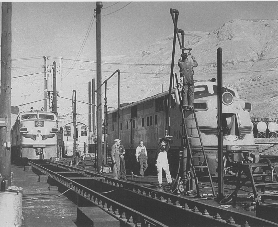
Workers adjust fueling devices in the "Goat Pit," an outdoor servicing area near the the Salt Lake City roundhouse, in December 1952. This area served as the diesel facility prior to the completion of the Salt Lake City Diesel Shops and was retained after its completion to service switch engines. Don Sims
