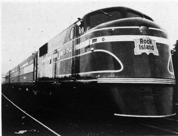
Above: Rock Island 'Rocket' train, one of the first to have a separate locomotive, in this case of Electro-Motive build and of 1,200 h.p.
