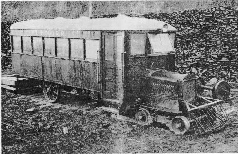
The third and last rail-auto used on the Mount Hood, probably the best and most used of the three machines. The body was constructed especially for the railroad and was mounted on a Mack truck frame. When it burned at Summit in 1935 it had traveled over 400,000 miles on a railroad less than 22 miles in length. Date of this picture is not known, but judging from the piles of cordwood in the background it was probably during the depression when Mount Hood locomotives were converted from oil to wood. (Courtesy of Donald C. Dietrich.)
