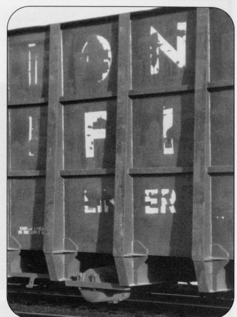
Left: This view shows the yellow end, rotary coupler and 38" wheelsets. Middle: The interior of the car is nothing more than a large "bathtub" with tapered sides. Right: Here's a closeup of the ribbing. Notice how the smaller horizontal ribs intersect the tapered vertical ribs. Channels extend under the car to support the bottom.
