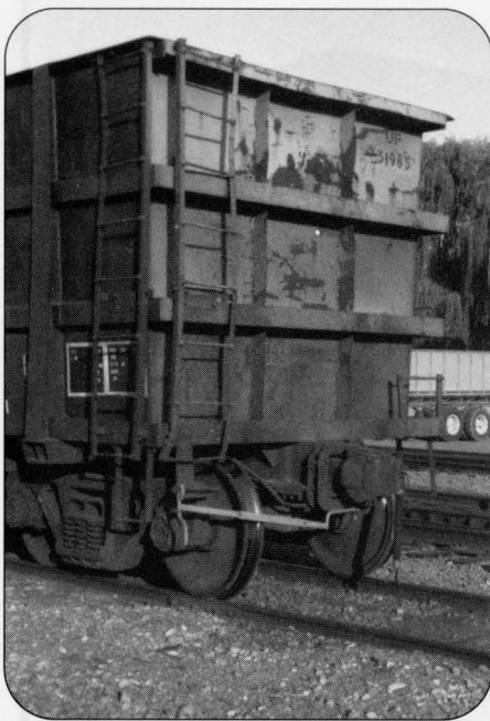
Left: This view shows the yellow end, rotary coupler and 38" wheelsets. Middle: The interior of the car is nothing more than a large "bathtub" with tapered sides. Right: Here's a closeup of the ribbing. Notice how the smaller horizontal ribs intersect the tapered vertical ribs. Channels extend under the car to support the bottom.
