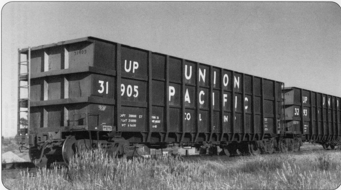
The Union Pacific "Coal Liner" has distinctive vertical and horizontal ribs and high sides. The ends of the car are painted yellow, indicating it's equipped with rotary couplers. Notice the large lettering between each of the ribs.
